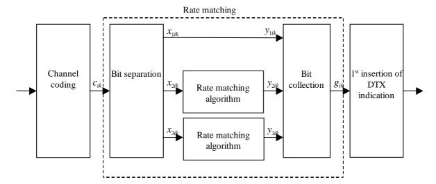
Figure 7: Puncturing of turbo encoded TrCHs in downlink
